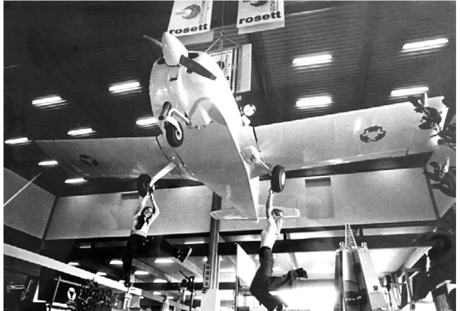
A one seater airplane with motor suspended from a shelving system (Elfa/Element) in 2 layers of 12 mm drywall fixed with Expandet Rosett. All loads are on the Rosetts! (±1970)
